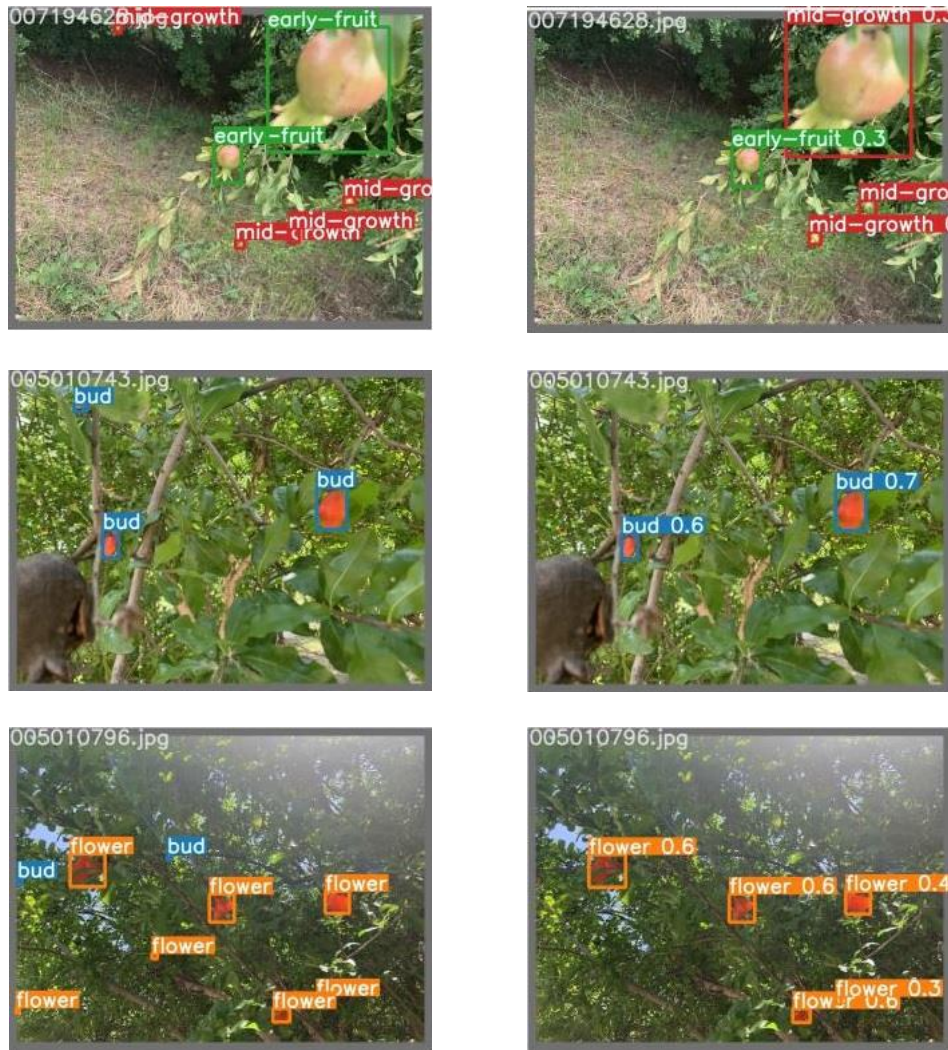
Figure 9. Test results of extreme early-fruit, flower and bud cases with ground truth (left) and predicted (right) labels
